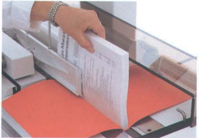
Release the bound book and place it on the heated tray for rapid drying.
