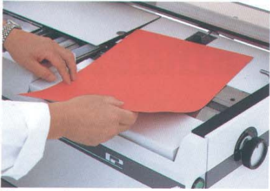
Take a cover from the top tray and align it to the three adjustable guiding points at the folding station.
