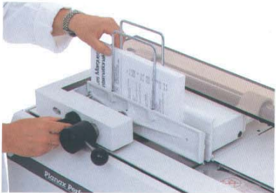
Set the material to be bound in the clamping station. Adjust the knob to the corresponding thickness and lock the turning handle.
