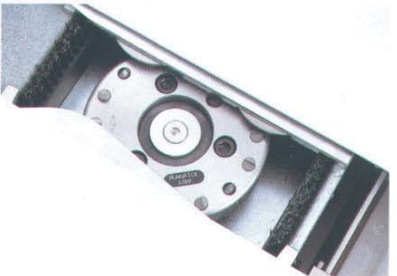
Combined milling and slitting head with exchangeable cutting metal tools.
